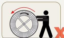
Drum shall not be rolled in the reverse direction.
