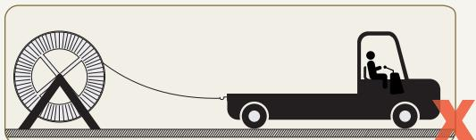
A convenient vehicle shall be used for pulling.
