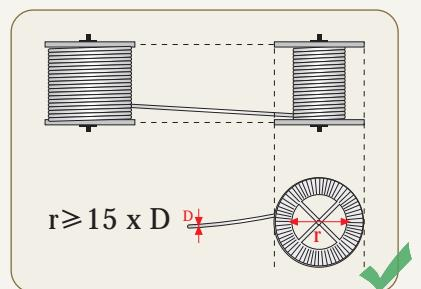
Center diameter of drum shall be arranged to cable size.
