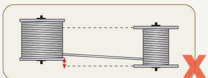
Centres shall be positioned horizontally equal during transfer.
