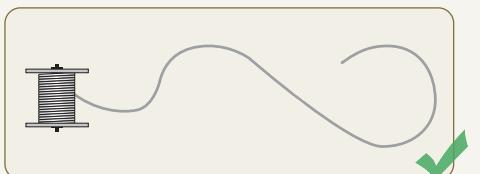
Minimum bending radius is important for uncoiling.
