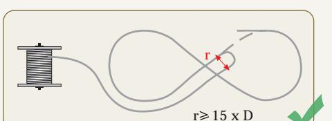
Minimum bending radius is important for uncoiling.
