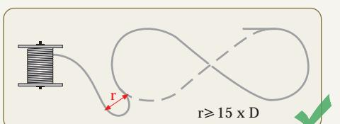
Minimum bending radius is important for uncoiling.
